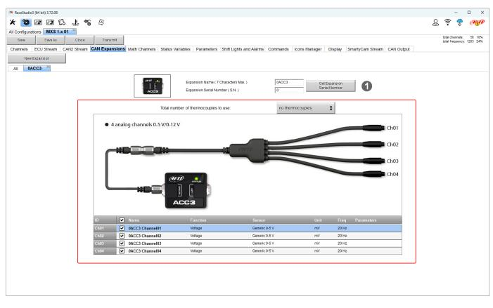
Select the cable in use, which strictly depends on the number of thermocouple sensors you plan to use. Make your selection in the **total number of thermocouples to use** (2 in the example).
