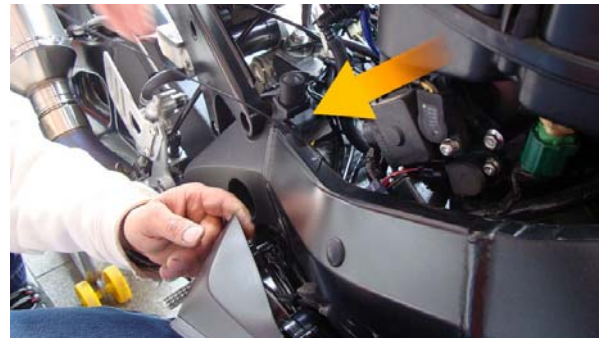
Figure 10: the ground cable runs along the chassis.
