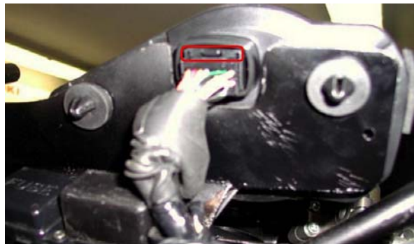
Figure 15: unplug the stock dash.
