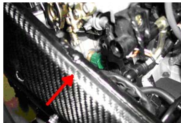
Figure 19: water temperature connector – particular.
