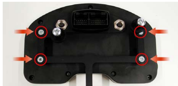
Figure 22 – MXL and bracket – rear view.
