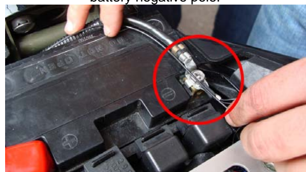
Figure 12: ground cable correctly connected.
