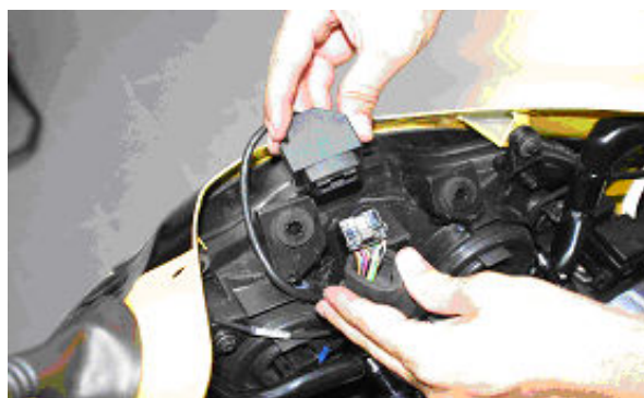
Figure 24 – wiring installation – particular of AMP connector.
