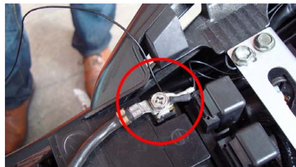
Figure 11: the connection of ground cable to the battery negative pole.
