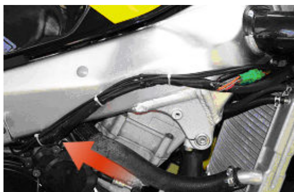
Figure 25 – wirings running along the bike chassis.
