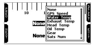
Each custom page can show up to four fields. Pressing "SELECT" you can choose the channel to show in each field. The only field that can show lap time in different formats is bottom right one (right image below).
