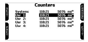
Each odometer can be activated or stopped and reset. Select the odometer you want to manage and press "CHANGE":
