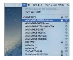
Verify that the status in the window that shows up is "Connected" and that the IP address associated is, for example, 10.0.0.10 (could be 10.0.0.11, 10.0.0.12, or generically 10.0.0.x).
