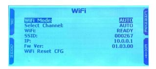
MyChron6 Wi-Fi configuration can be made only using Race Studio 3 software. Two possible Wi-Fi modes are available:
