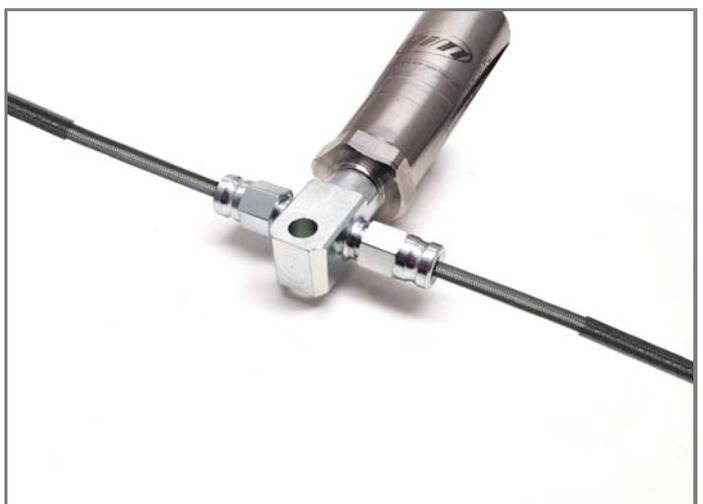
**Warning:** once the installation is over ensure that the brake circuit is cleared and check its tightness.
