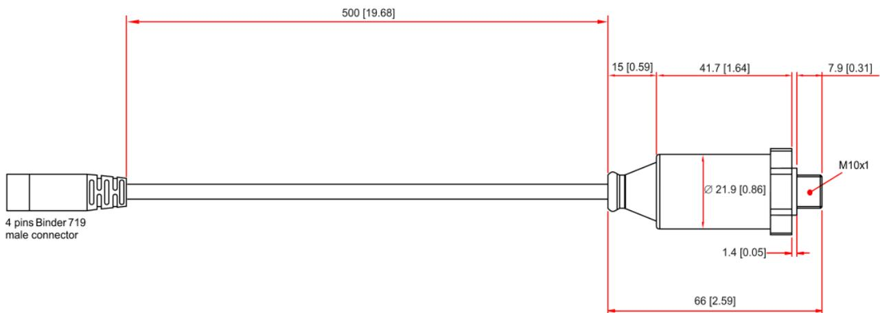
The sensor ends with a 4 pins Binder 719 male connector. The image below shows the connector pinout from solder termination side.
