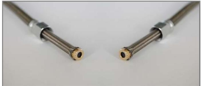
Press the nipple until the contact with the internal part of the pipe ("A") is complete and then cover it with the metallic braid.
