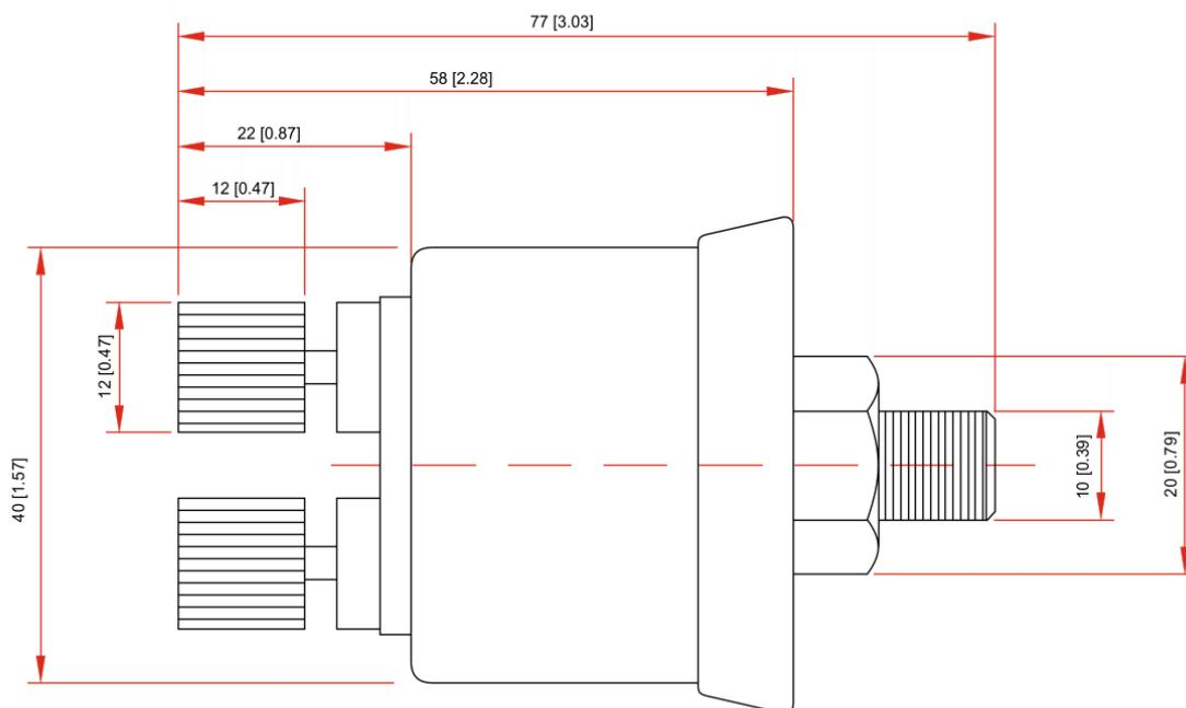
The drawing below shows VDO cable dimensions in millimetres [inches].
