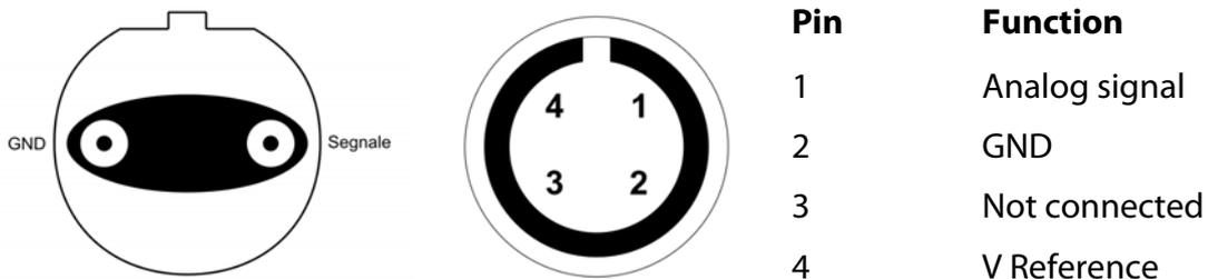
The table here below shows the sensor electrical characteristics.
