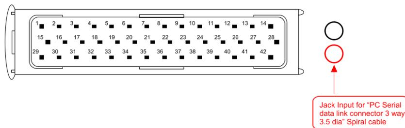
The ECU comes with a spiral cable ending with a Jack on one side and alternatively a DB9 female or a DB25 female on the other side. The Jack input of the ECU to be used is shown here above. The spiral cable is used to program the ECU as well as to communicate with external devices, like AIM ones. Here below the spiral cable ending with a DB9 female connector is shown.
