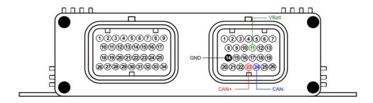
The ECU communicates through the CAN bus on the 26 pins connector. This ECU needs GND and Vbatt connection too. Please refer to your AIM device pinout to connect them. ECU connectors pinout and connection table are shown below.
