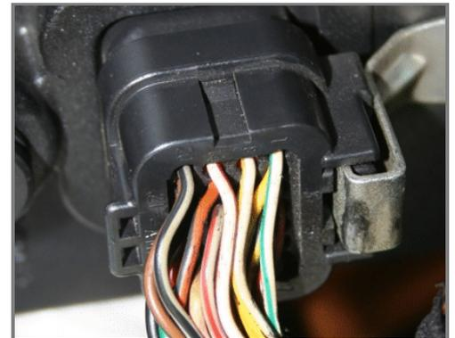
To connect AiM devices to Ducati ECU through the dashboard use its 26 pins rear connector. Here below are its pinout and the connection table.
