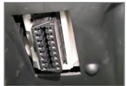
The ECU communicates using the K line on the OBDII connector. Connector pinout as well as connection table are shown here below.
